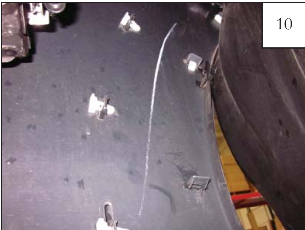
Using a flat head screwdriver, with a pressing motion, remove eight plastic clips located inside of bumper cover. Remove front flare bumper extension.
