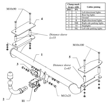
This towbar is designed to assembly in following cars: OPEL ASTRA "G" 4 door, produced since 10.1998 and OPEL ASTRA "G" 3/5 door, produced since 03.1998, catalogue no. E21A and is prepared to tow trailers max total weight 1500 kg and max vertical load 75 kg.
