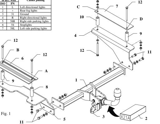
This towing hitch is designed to assembly in following cars: CHEVROLET AVEO SEDAN, produced since 2006 till 2011, catalogue no. X21A and is prepared to tow trailers max total weight 1200 kg and max vertical mass 75 kg.
