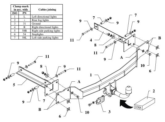
This towing hitch is designed to assembly in following cars: **MERCEDES S-CLASS** produced since 1999 till 2005, catalogue no. **D36A** and is prepared to tow trailers max total weight **2100 kg** and max vertical load **85 kg**.
