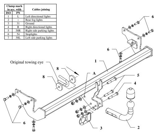
This towbar is designed to assembly in following cars: MITSUBISHI SPACESTAR, produced since 06.1998 till 12.2004, catalogue no. Z16 and is prepared to tow trailers max total weight 1400 kg and max vertical load 75 kg.
