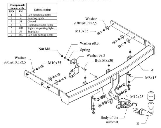
This towbar is designed to assembly in following cars: **FORD GALAXY** produced since 1995 till 05.2000; **VW SHARAN** produced since 1995 till 04.2000; **SEAT ALHAMBRA** produced since 1996 till 04.2000, catalogue no. **C33A** and is prepared to tow trailers max total weight **2100kg** and max vertical mass **85kg**.
