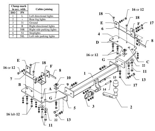
This towing hitch is designed to assembly in following cars: **TOYOTA LANDCRUISER (J100),** produced since 1998 till 12.2002, catalogue no. **O35** and is prepared to tow trailers max total weight **3500 kg** and max vertical load **120 kg**.
