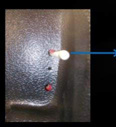
Outer holes can be used as guide to cut a 3/4" circular holes. <u>Tie-down has to</u> <u>be removed and</u> <u>re-installed over</u> <u>the Bedliner</u> OPTIONAL INSTALLATION KIT, PART NUMBER = LIK 34 (sold separately)
