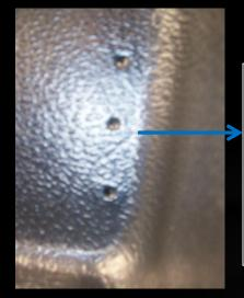
Center hole can be used as guide to cut a  $2\frac{1}{2}''$ circular hole to expose tie-down front or rear.
