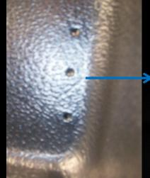
Center hole can be used as guide to cut a 2 <sup>1</sup>/2" circular hole to expose tie-down front or rear.
