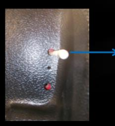
Outer holes can be used as guide to cut 3/4''circular holes. <u>Tie-down has to</u> be removed and re-installed over the Bedliner
