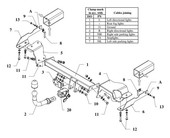
This towbar is designed to assembly in following cars: **Toyota Yaris CP10** (**Japanese version**), produced since 1999 till 2001 and **Toyota Yaris CP10** (**French version**), produced since 2002 till 2005, catalogue no. **O24A** and is prepared to tow trailers max total weight **900 kg** and max vertical load **50 kg**.
