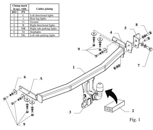
This towbar is designed to assembly in following car: **NISSAN ALMERA, 3/5 door, (N16),** produced since 03.2000 till 2006, catalogue number **V49A** and is prepared to tow trailers max total weight **1500 kg** and max vertical load **75 kg**.
